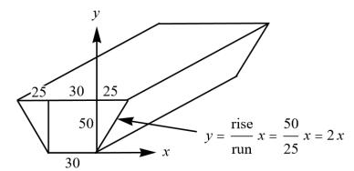
The aim is to find the volume V(y) that water occupies if it's at a height y. In order to do this, find the area of a cross-section and then multiply it by 10 meters (1000 centimeters), the thickness.
